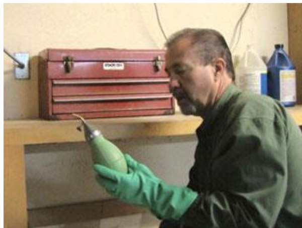
Using a hand duster to apply tracking powder
