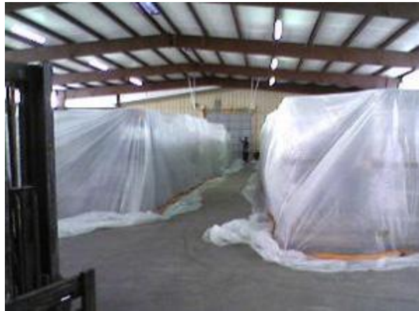
Fumigation on impermeable surface (photo: pestcontrolcape.co)
